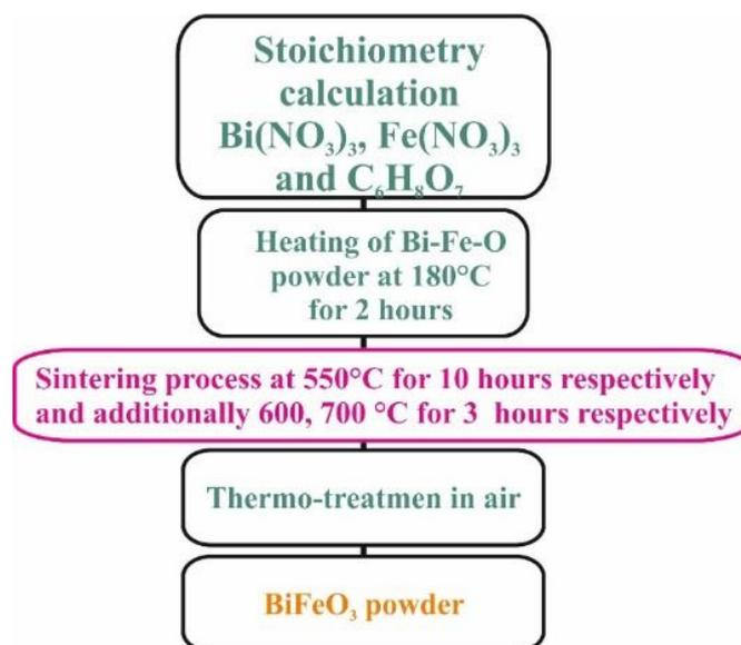
**Fig. 1.** The main stages of sol-gel synthesis of BiFeO<sub>3</sub> powders.
