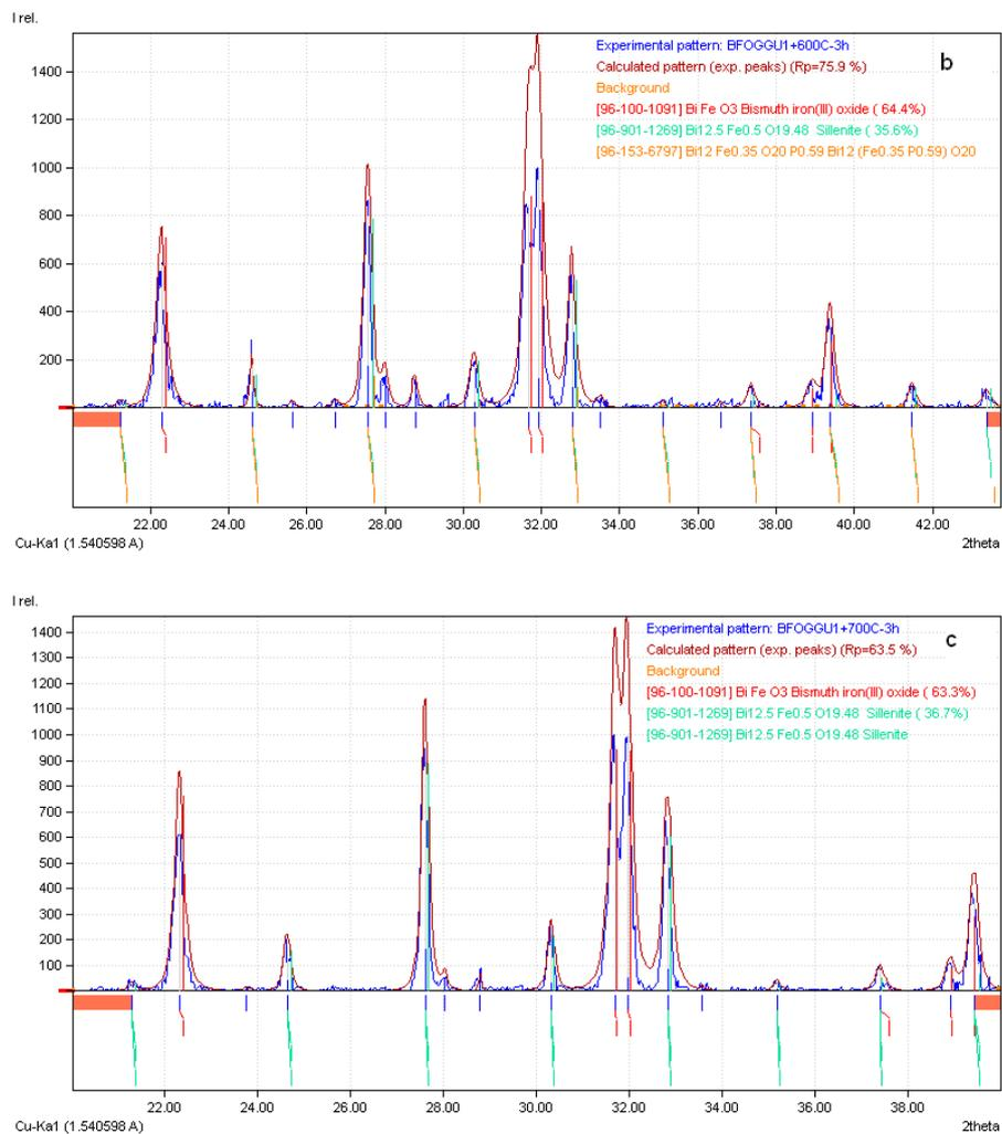
**Fig. 3.** XRD of  $\text{BiFeO}_3$  powder obtained by sol-gel method.
