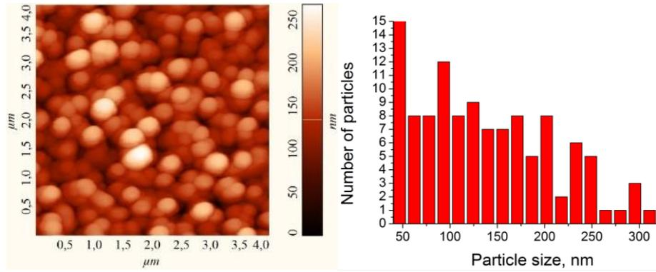
**Fig. 2.** AFM-image of BiFeO<sub>3</sub> powder obtained by sol-gel method (annealing temperature 550 °C ) – left image. Particle distribution graph is denoted on the right image.
